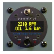
Additional multi-display modes are user selectable and enable the Status Monitor to become a simple digital RPM meter or to indicate MAP, Oil Pressure and Coolant Temperature. These modes are particularly useful when the unit is being used as an EMS backup or as the sole instrument during initial engine start and tests.
