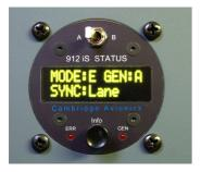
For example and as shown here (left), generator and engine mode information is available at the press of a button.
