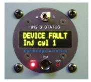
In the event of an ECU Lane problem (or Lane lamp illuminating) the Status Monitor immediately indicates the failure and provides a readable description of the problem (example shown left).
