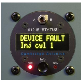
In this example, a device fault is being indicated by Lane B.
