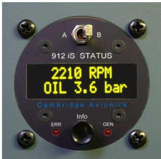
Typical displays when Multi-Display is enabled with the '+MAP/O/C met' option and Lane B selected.
