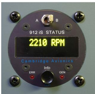
A typical display when Multi-Display is enabled with the 'RPM Only' option.
