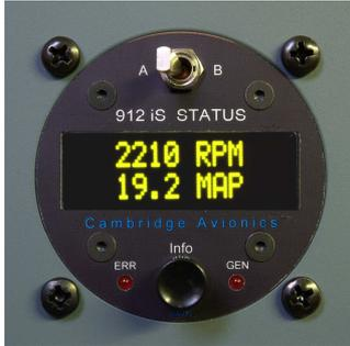
A typical display when Multi-Display is enabled with the '+MAP/Oil imp' option and Lane A selected.
