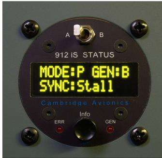
For example, this is typically what is seen prior to engine start when monitoring the Lane A CANbus.
